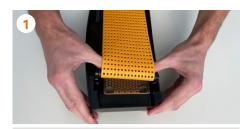
Place the PulpOut system on a smooth surface, place your fingers on the inside of the **sweeping belt roller** and push it outwards to release it.
