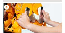
Remove 1Step Extraction kit and the blade.
