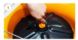
Remove the **feeder plate** by unscrewing the central knob.
