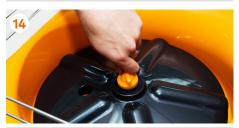
Insert the **feeder plate** by screwing the central knob.
