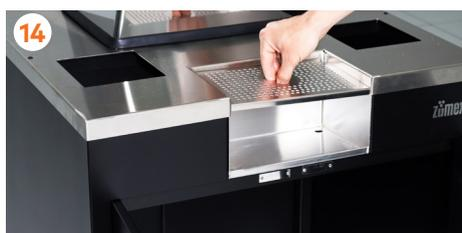
14 Clean the inside of the **podium**, following the steps shown and removing all the particles which have adhered.
