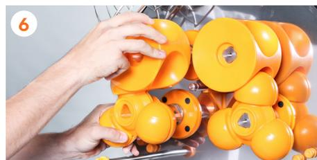
6 Unscrew the securing knobs of the pressing units. Take off the pressing units in pairs.
