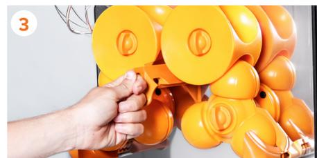
3 Remove the **blade** by pressing on the centre and pulling the handle towards you.
