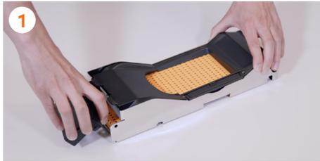
**1** Rest the PulpOut system on a flat surface and disassemble the **side cover**, holding it from above to remove the ends of the guides.
