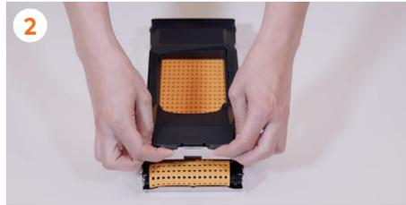
**2** Remove the black **upper lid** by pushing upwards on the tabs sticking out.
