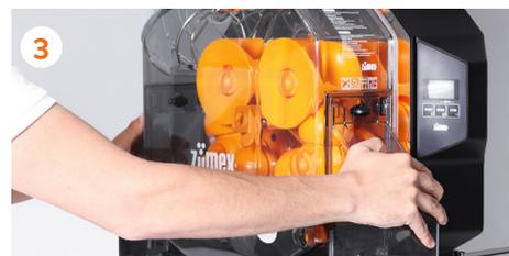
3 Turn the knobs and take off the **front cover** as well as the side outputs.
