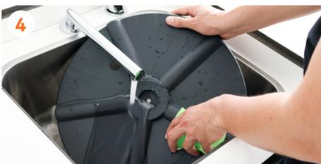
Wash the **feeder plate** with Citric Active and a soft sponge, removing all the particles which have stuck to it.
