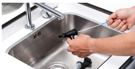
Dose the degreaser by inserting the spray nozzle into the three orifices and applying the product. Scrub the inside through the holes with the aid of the small brush supplied.
