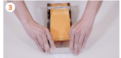
**3** Turn the assembly around and place your fingers on the **sweeping belt** by pushing it outwards to release it.
