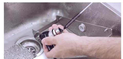
Rinse with water, apply the disinfectant, rinse again and to finish, dry both the outside and the inside of the tap with paper (roll the paper on the pin to aid insertion of the paper into the holes).
