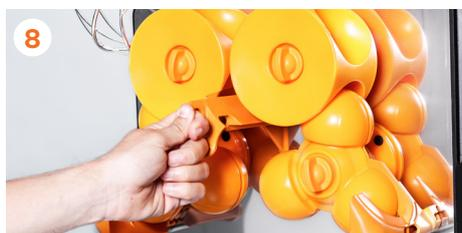
8 Remove the **blade** by pressing on the centre and pulling the handle towards you.
