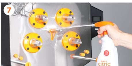
7 Clean the front zone of the machine, following the steps shown and removing all the particles which have adhered.
