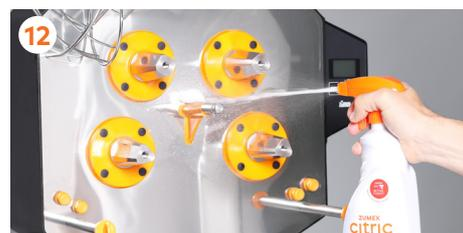
12 Clean the front zone of the machine, following the steps shown and removing all the particles which have adhered.
