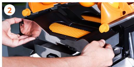
2 Take off the **automatic PulpOut System**, by lifting the assembly with the part closest to you.
