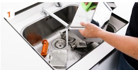
Follow the cleaning process indicated, for all the parts: **blade, sub-filter, tank, peel chutes**, etc.
