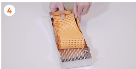
**4** Remove the **sweeping belt** together with the other roller and remove both parts.
