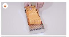
Remove the **sweeping belt** together with the other roller and remove both parts.
