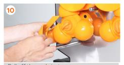
Pull off the peel ejectors.
