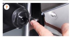
Press the side tabs to remove the **bin**.
