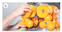
Unscrew the securing knobs of the pressing units. Take off the pressing units in pairs.
