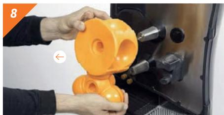
8 Remove both the upper and lower securing knob.
