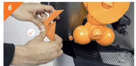
6 Remove the peel ejector pulling sideways.
