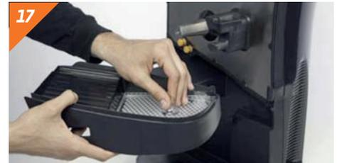
17 Place the filter in its correct position.
