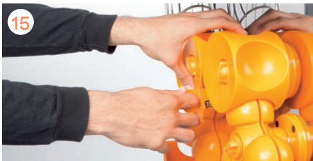
Put on the knife. Push until it clicks into place with a "clac"
