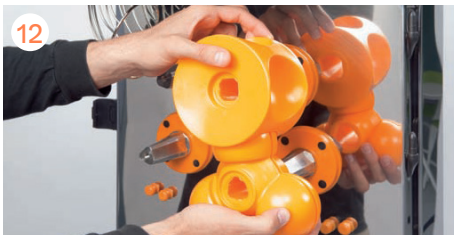
Mount the pressing units by pairs.
