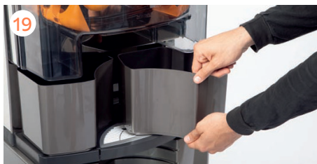
Place the peel buckets.
